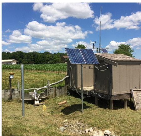
You've probably seen one of these, a field water quality sampling station and on-line weather station.
